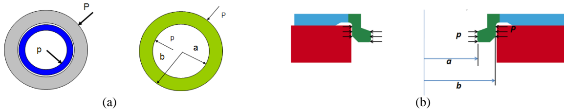
Figure 4: (a) Swaging schematic (b) Arm aperture model as thick cylinders
