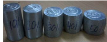
Fig.2.(f): Al-10Si-10%TiB 2 composite specimens showing bulge profiles at various deformation stages under compression testing at aspect ratio 1.5.
