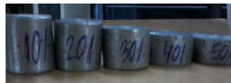
Fig.1(c): Al-10Si-4%TiB 2 composite specimens showing bulge profiles at various deformation stages under compression testing at aspect ratio 1.
