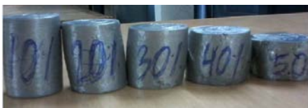
Fig.2.(c): Al-10Si-4%TiB 2 composite specimens showing bulge profiles at various deformation stages under compression testing at aspect ratio 1.5.
