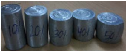
Fig.2.(a): Al-10Si alloy specimens showing bulge profiles at various deformation stages under compression testing at aspect ratio 1.5.
