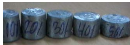
Fig.1(b): Al-10Si-2%TiB 2 composite specimens showing bulge profiles at various deformation stages under compression testing at aspect ratio 1.0.
