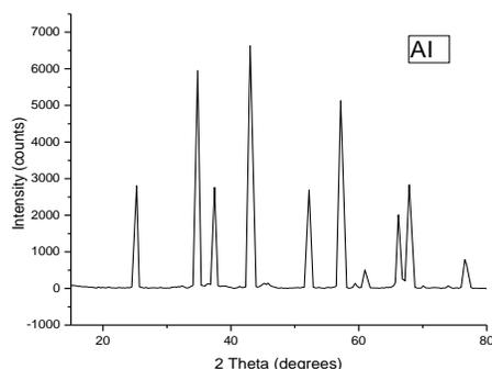
Figure 1(a) XRD pattern of nano  $\text{Al}_2\text{O}_3$  without PVA
