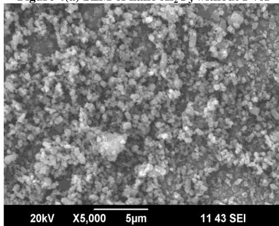
Figure 4(b) SEM of nano Al<sub>2</sub>O<sub>3</sub> with PVA
