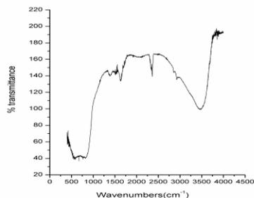
Figure 2(a) FTIR spectrum of nano Al<sub>2</sub>O<sub>3</sub> without PVA
