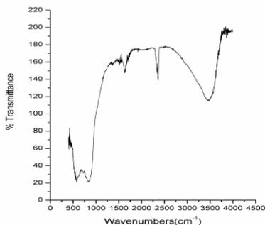
Figure 2(b) FTIR spectrum of nano Al<sub>2</sub>O<sub>3</sub> with PVA
