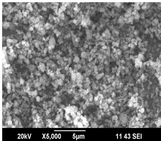
Figure 4(a) SEM of nano Al<sub>2</sub>O<sub>3</sub> without PVA
