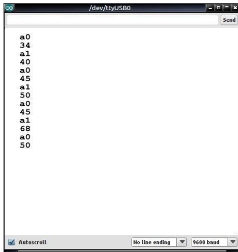
fig3.1 Arduino Reading of Case-1 a0- Reading of IR sensor-1 a1- Reading of IR sensor-2
