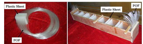
Fig: 02. Form-work of wood and thermocol
