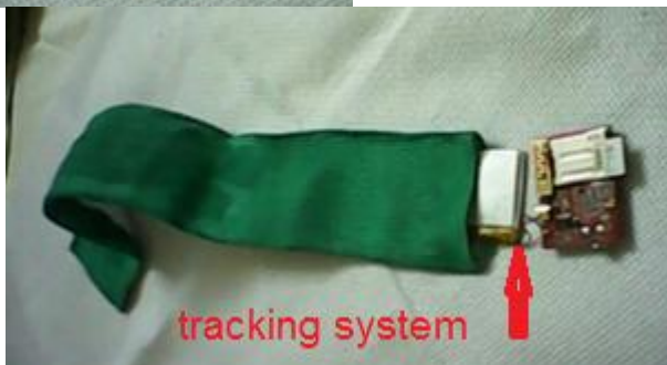
Figure No7 showing the tracking system inside the belt.
