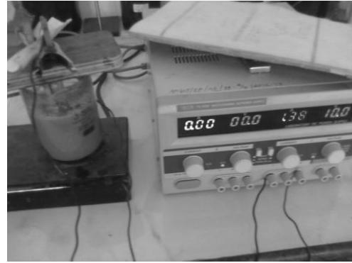
Fig-1: Bench-scale EC reactor with monopolar electrodes
