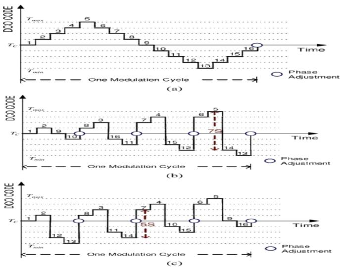
Fig. 2(a) illustrates the conventional triangular modulation with digital approach [9]. Since the output frequency can be changed by the DCO control code, the output clock frequency
