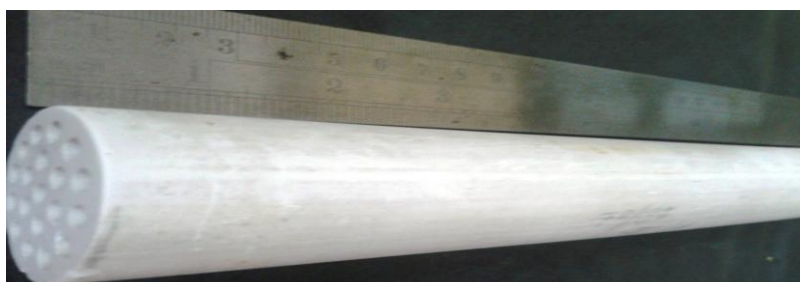
Figure 2: Configuration of low cost alumina based tubular 19-channel MF membrane element of 1 meter length.
