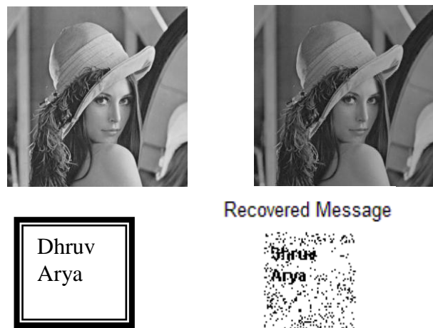
Fig.5 DCT Domain Watermarking Technique going from Top Left to Right A. Original Image B. Watermarked Image C. Watermark D. Extracted Watermark
