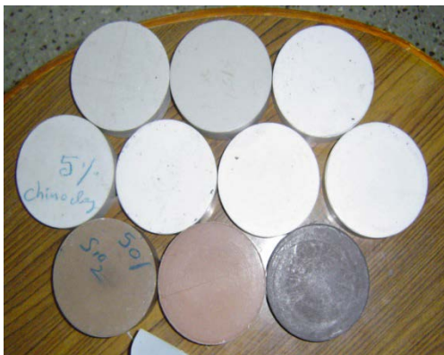
Photograph2: Virgin PTFE and its filled composite billets- before and after sintering including skiving tapes.
