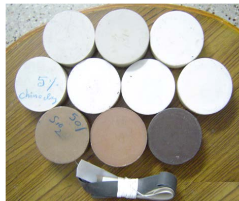
Photograph2: Virgin PTFE and its filled composite billets- before and after sintering including skiving tapes.
