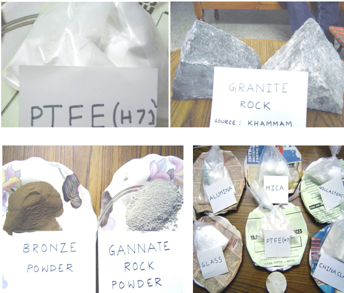
Photograph 1: Virgin PTFE and different fillers used.
