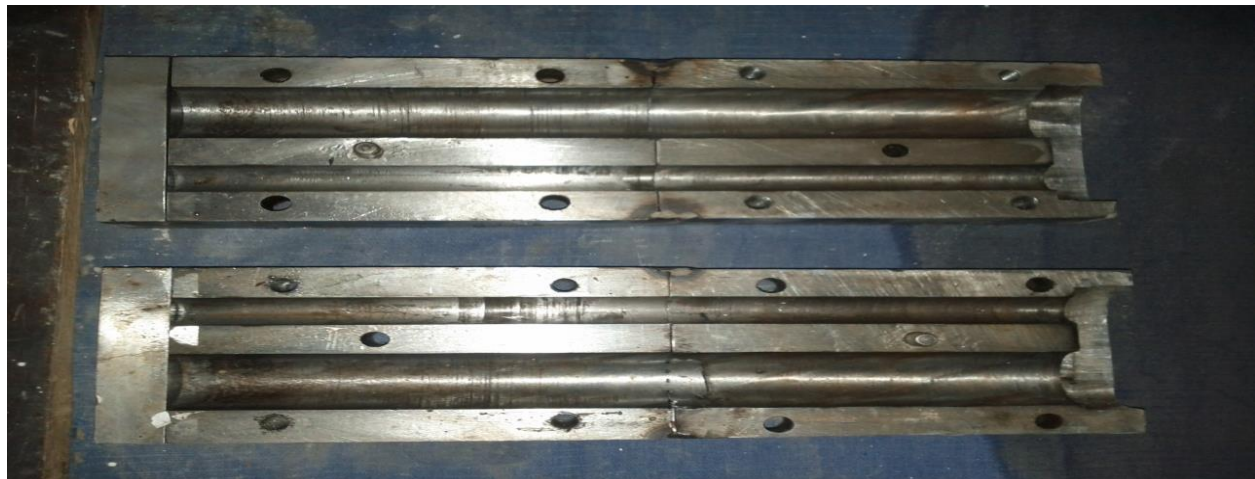
Fig.2- Die for casting of samples for wear test
