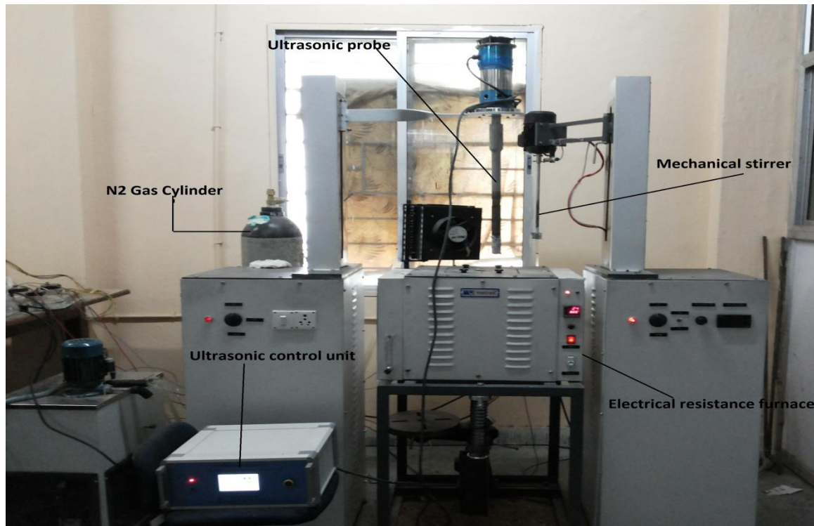
Fig. 1 Ultrasonic assisted stir casting setup
