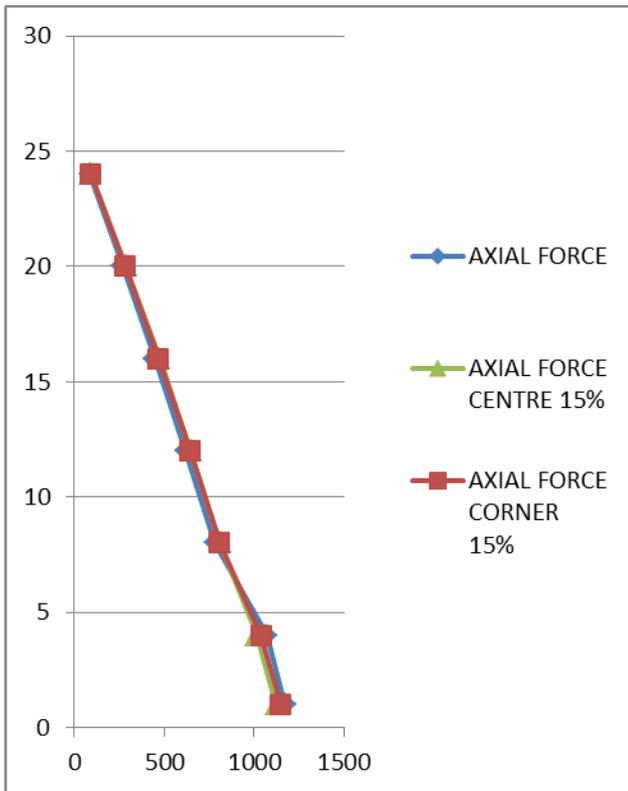
**Fig 7.2: Axial Force in (kN) for column No. 1**
