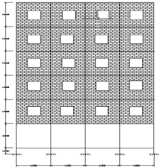
**Fig6.3; MODEL III: INFILLED FRAME WITH CENTRE OPENING**
