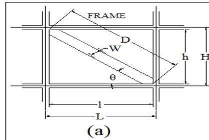
Fig.1 Brick Infill Panel as Equivalent Diagonal Strut
