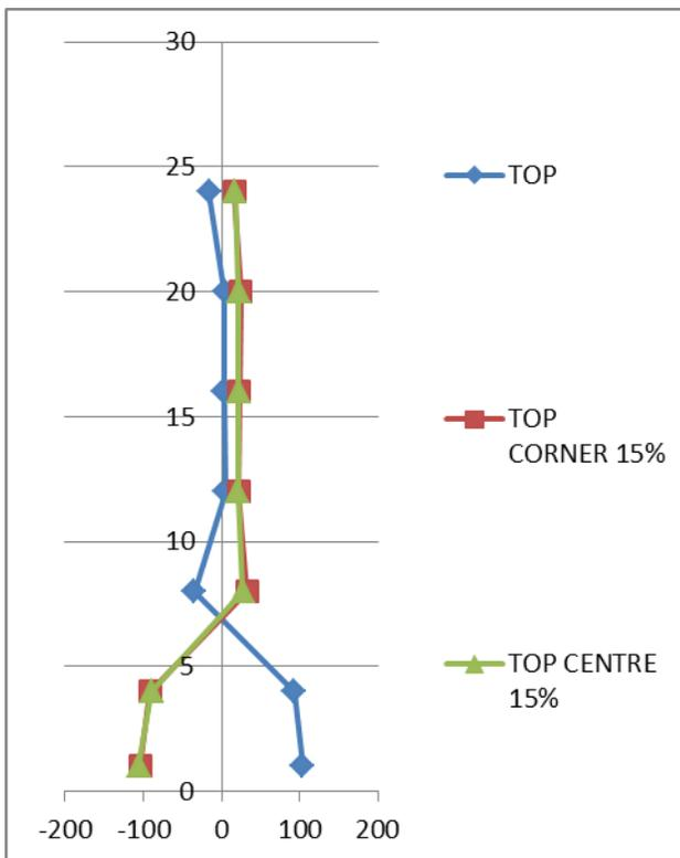
**Fig7.3: B.M (Top) in (kN-M) for column No.1**
