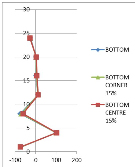
Fig 7.9: B.M (Bottom) in (kN-M) for column No.2
