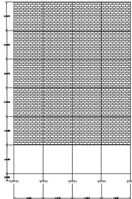
Fig6.2; MODEL II: WITH FULLY INFILLED FRAME
