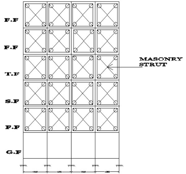
**Fig6.5; EXAMPLE OF STRUT FRAME MODEL**
