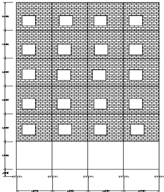
**Fig6.4; MODEL IV: INFILLED FRAME WITH CORNER OPENING**
