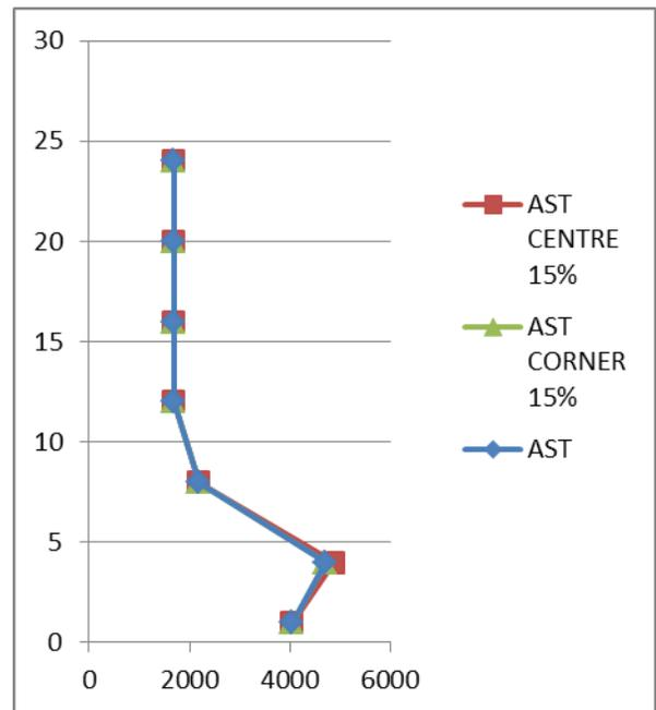
**Fig7.5: Area of steel in (mm2) for column No.1**
