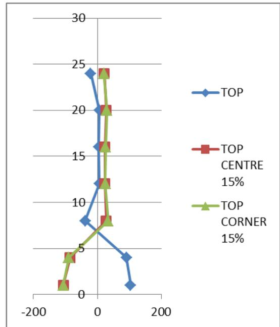
Fig 7.8:B.M (Top) in (kN-M) for column No. 2
