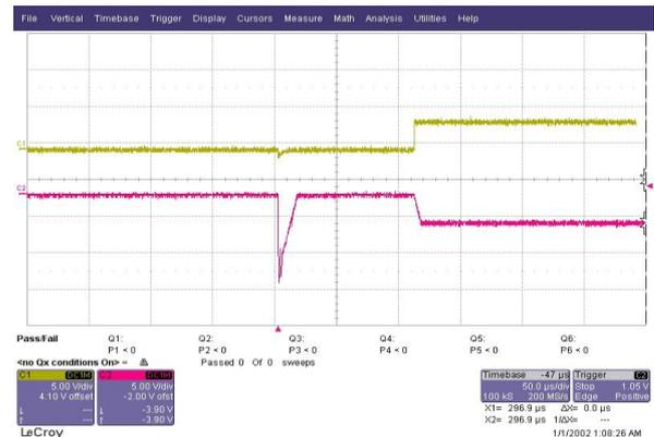
Figure 5: Output after a discharge of 15kV at a distance of 0.7m
