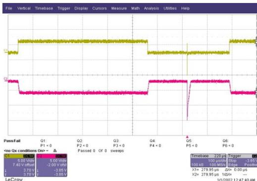
Figure 3: Output after a discharge of 4kV at a distance of 0.7m
