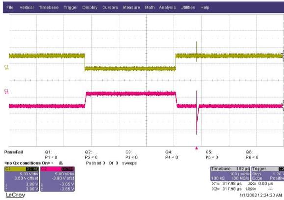
Figure 6: Output after a discharge of 4kV at a distance of 0.9m
