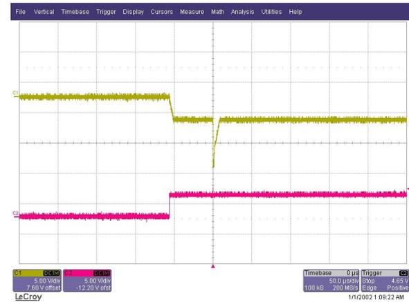
Figure 10: Output after a discharge of 12kV
