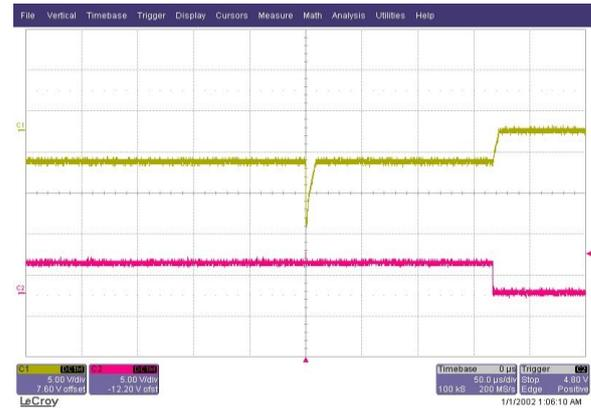
Figure 9: Output after a discharge of 8kV
