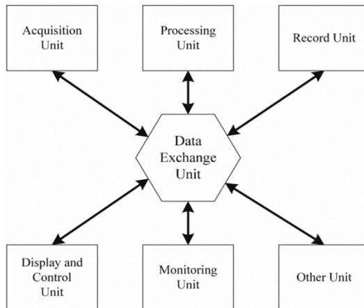
Fig.1. Block diagram of radar signal processing system based on data exchange
