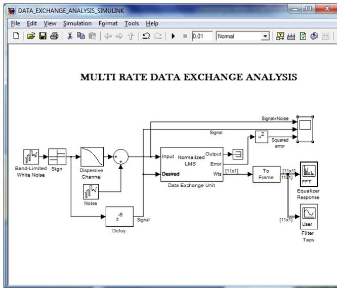
Fig.5. SIMULINK Model for Multi Rate Data Exchange Analysis
