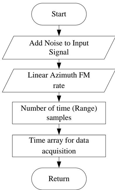
Fig.3. Sub Function of System Flowchart
