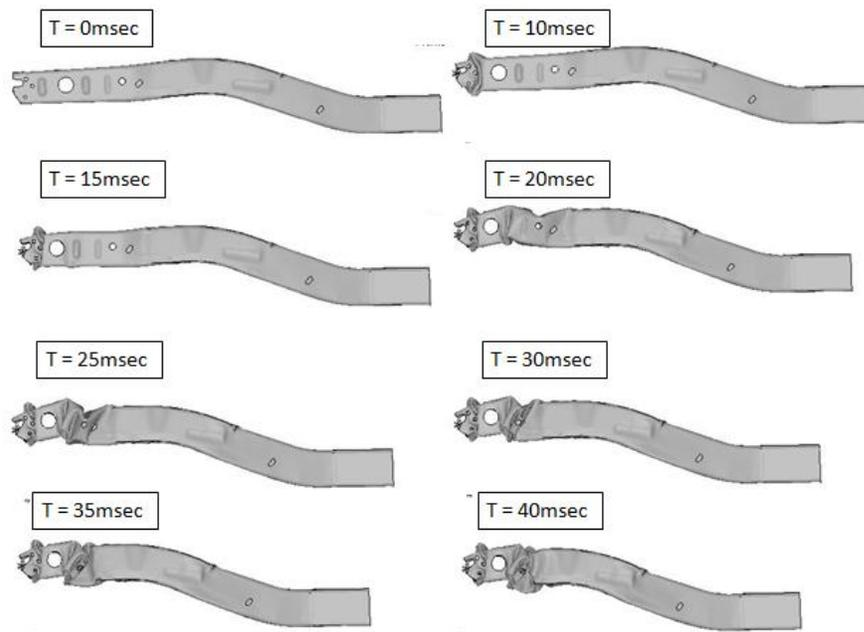
This is the front longitudinal member for which material is varied to study the effect of material yield strength. This member is deformed during the crash event initiating a collapse at 25 milliseconds. Maximum resistance is offered before the collapse is function of thickness, geometry and material.
