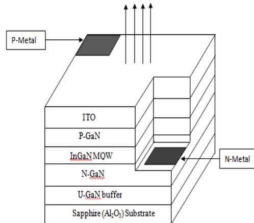
Figure 1: Basic Structure of 550 nm LED.
