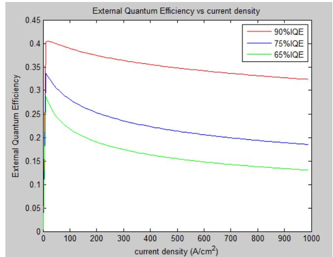
Figure 4: External Quantum Efficiency vs Current Density curve.
