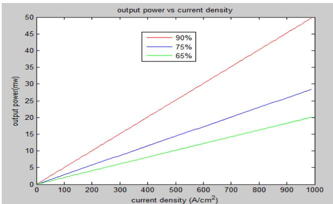
Figure 3: Output power vs Current density curve of Green LED.
