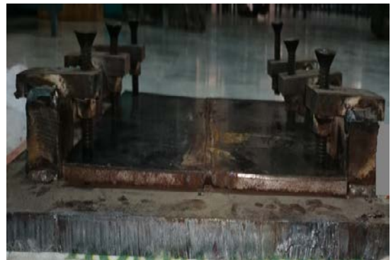
Figure 14: Image of Normal Welding of 8mm Thick Plates with Fixture
