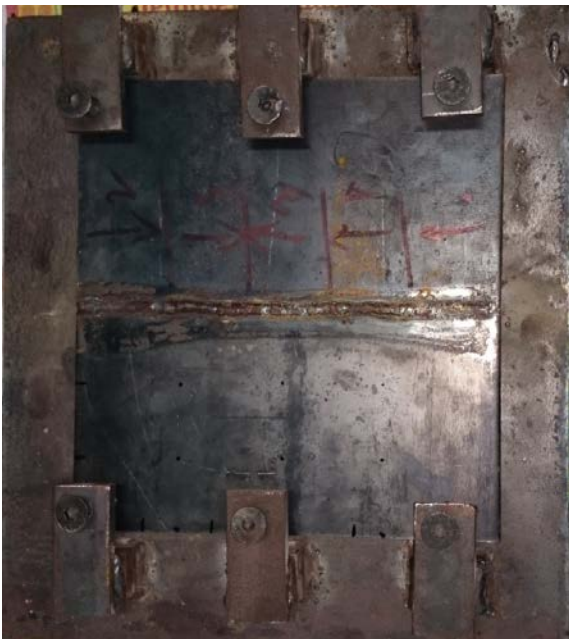
Figure 4: Image of Normal Welding of 4mm thick Plates with Fixture
