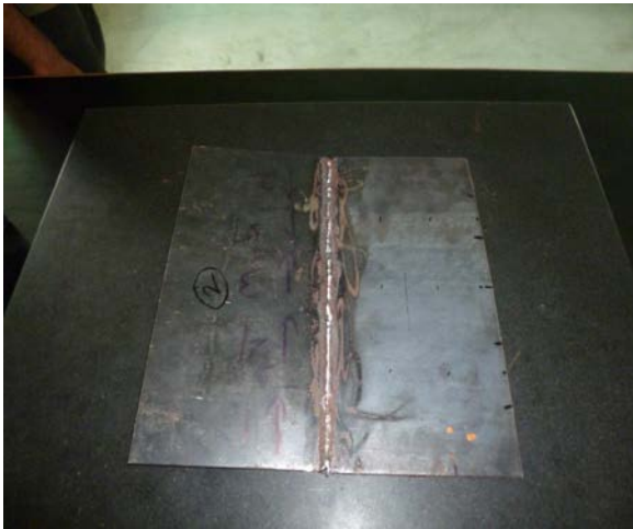
Figure 11: Normal Welding of 8mm thick Plates
