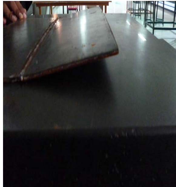
Figure 13: Distortion of 8mm Thick Plates in Normal Welding
