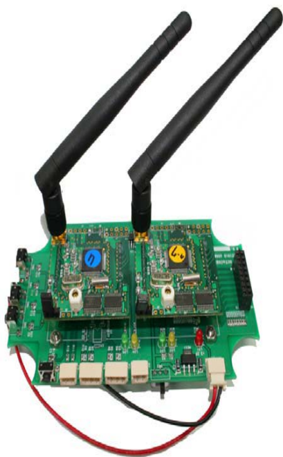
Figure 3. Developed interface board and RF board
