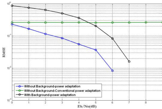
**Fig.5 Plot Showing RMSE values of Proposed, Conventional Power methods with and without background**
