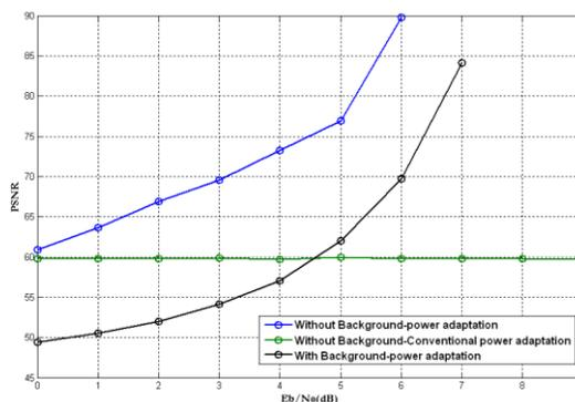
Fig.4 Plot Showing PSNR values of Proposed, Conventional Power methods with and without background
