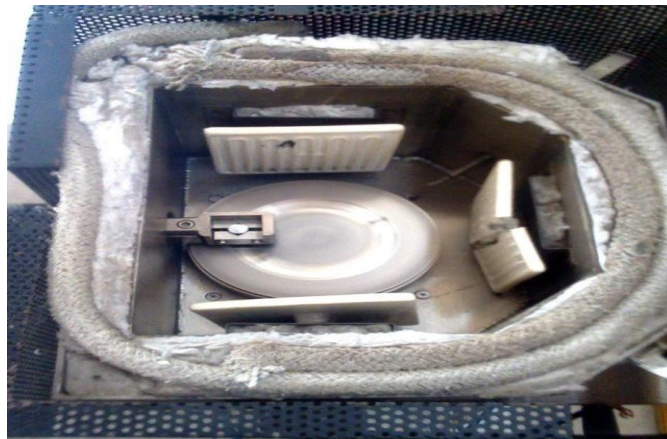
Fig. 2 Pin on Disc wear testing machine TR20CH
