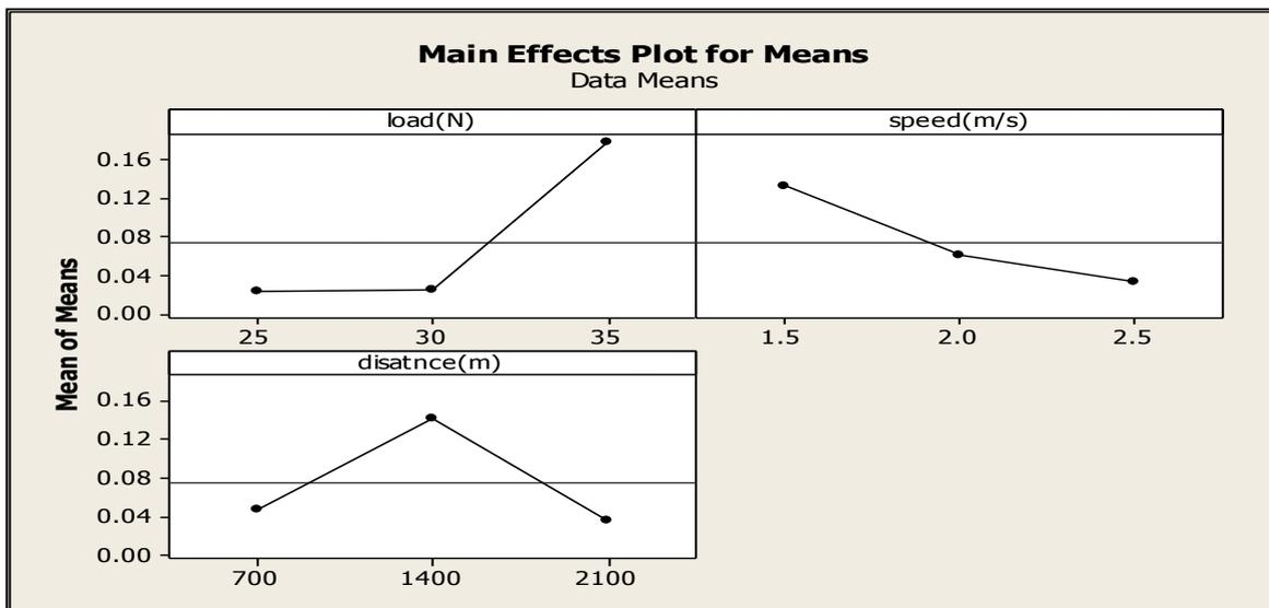
**Fig. 4- Main Effects Plot for Means-Wear rate**
