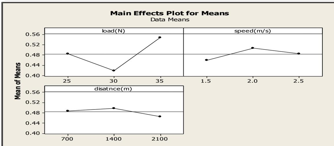
**Fig.6-Main Effects Plot for Means-coefficient of friction**
