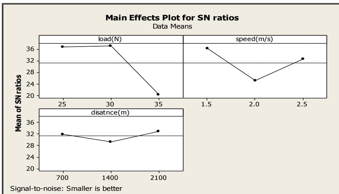
**Fig. 3-Main Effects Plot for SN ratios-Wear rate**
