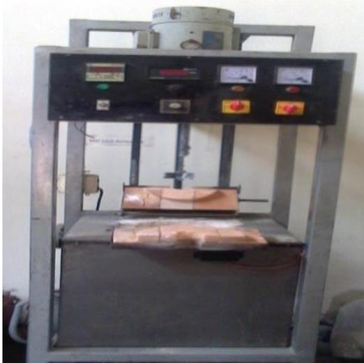
Fig.1 Stir Casting Setup
