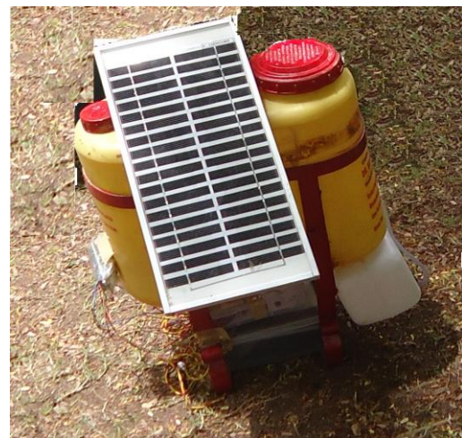
Figure 3: Working model of multiple power supplied fertilizer sprayer
