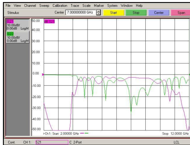
Figure 2. Measured results of reflectance and transmittance of a single ring microstrip filter
