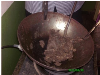
Figure: 3 manual hot mixing of jute with pp
