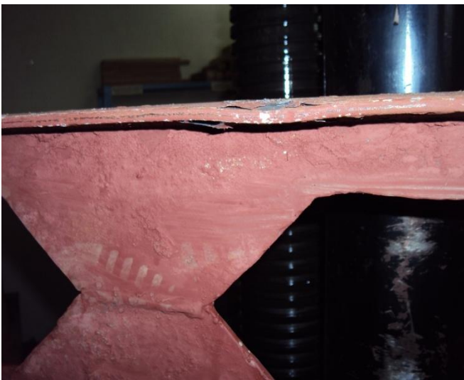
Fig.4 Local Failure Mode -Buckling of Compression Flange
