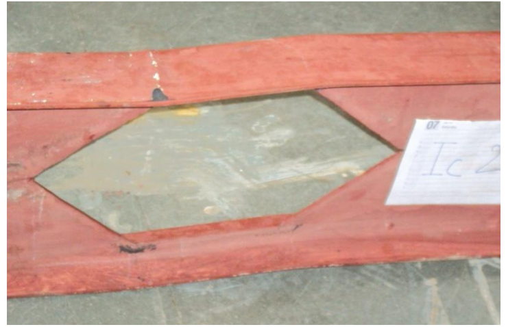
Fig.6 Stress Concentration in Ic 225 at Hole Corner
