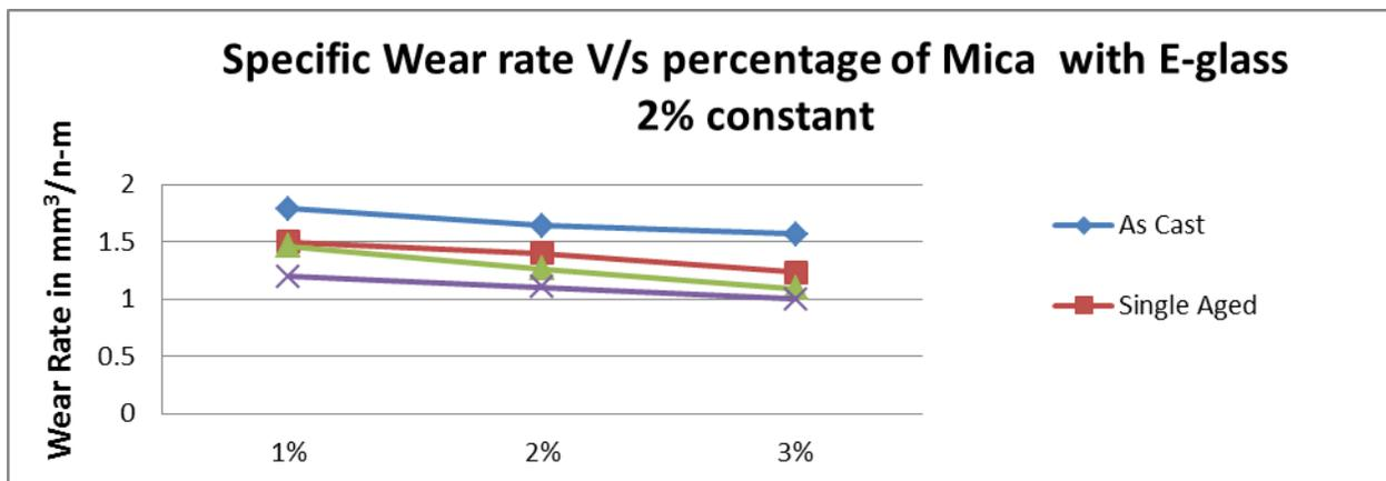
**Graph 5. Shows Evaluation of Specific wear rate for samples with various Mica Compositions and aging conditions with E-glass 2% constant**
