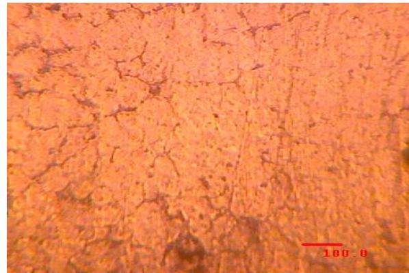
**Fig3: Microstructure of Single aged Al6061 Composite (2wt% mica, 2wt% E-glass fiber)**
