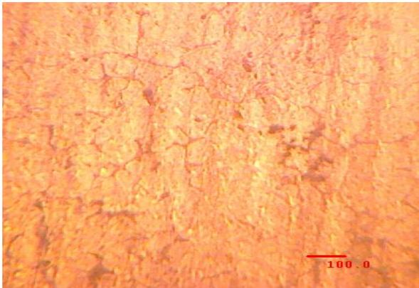
**Fig2: Microstructure of As-Cast Al6061 Composite (2wt% mica, 2wt% E-glass fiber)**
