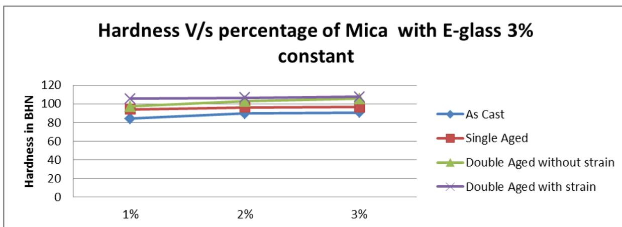
Graph 3. Shows Evaluation of hardness for samples with various Mica Compositions and aging conditions with E-glass 3% constant
