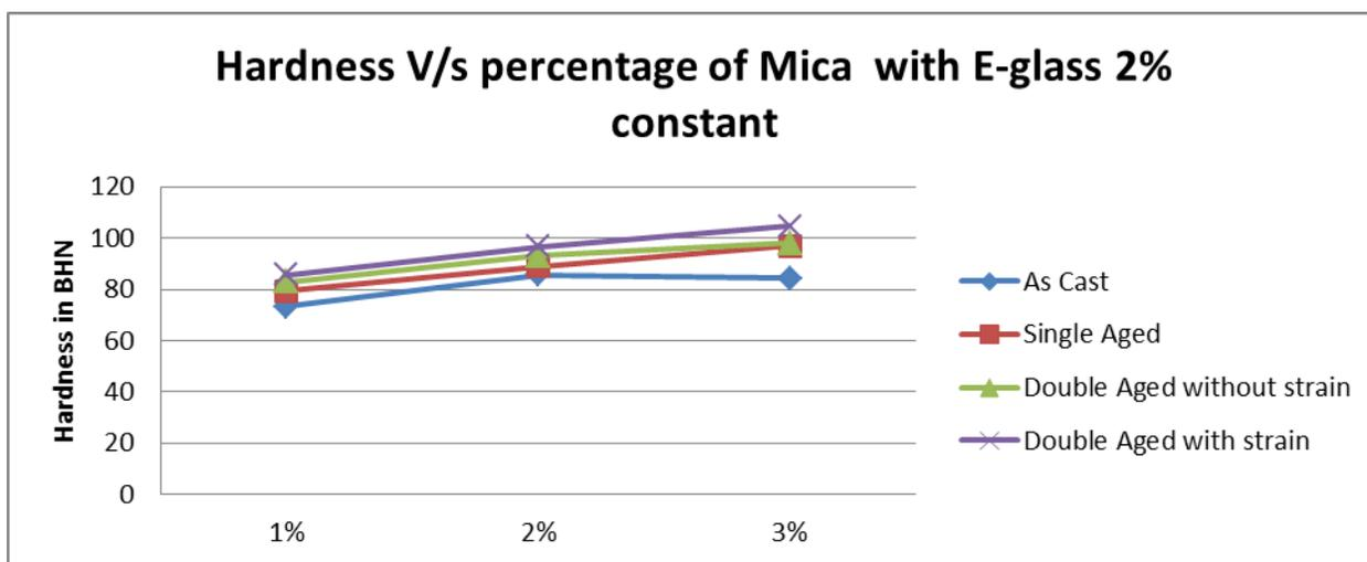
Graph 2. Shows Evaluation of hardness for samples with various Mica Compositions and aging conditions with E-glass 2% constant
