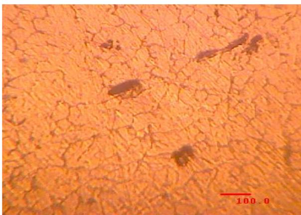
**Fig4: Microstructure of Double aged without strain Al6061 Composite (2wt% mica, 2wt% E-glass fiber)**
