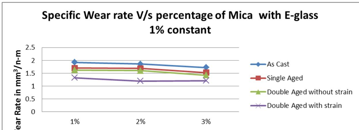
**Graph 4. Shows Evaluation of Specific wear rate for samples with various Mica Compositions and aging conditions with E-glass 1% constant**
