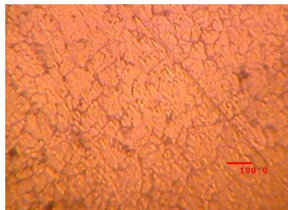
**Fig5: Microstructure of Double aged with strain Al6061 Composite (2wt% mica, 2wt% E-glass fiber)**
