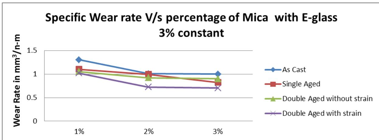
**Graph 6. Shows Evaluation of Specific wear rate for samples with various Mica Compositions and aging conditions with E-glass 3% constant**
