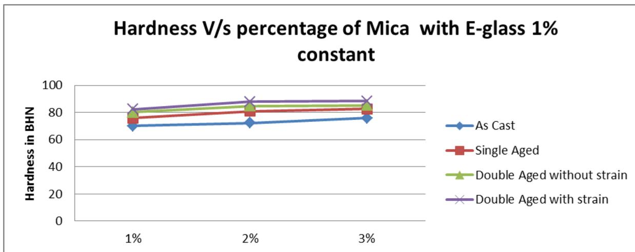
Graph 1. Shows Evaluation of hardness for samples with various Mica Compositions and aging conditions with E-glass 1% constant
