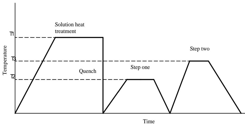
**Fig. 1: Schematic representation of temperature Vs time plot showing both solution and precipitation heat treatments (artificial ageing).**
