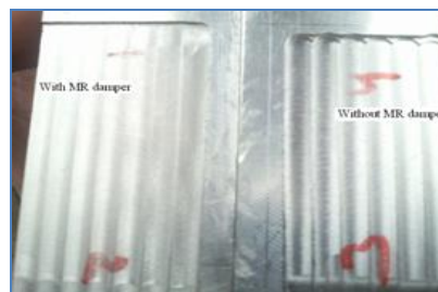
Fig 5: Chatter marks on the machined surface
