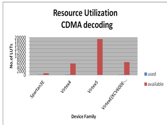
Fig.7.b. Resource Utilisation performance of CDMA Decoding
