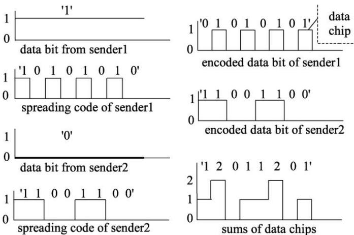
**Fig.4. CDMA Encoding using Code words of Length 8**
