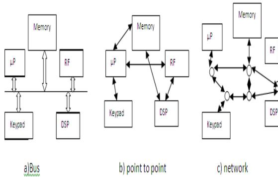
**Fig.1 On chip Communication Architecture**
