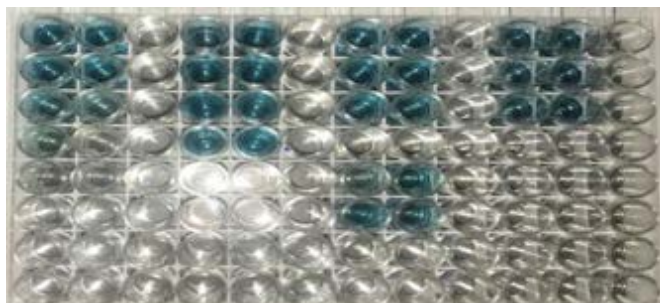
Figure 4: The color reagent is added to each well after wash
