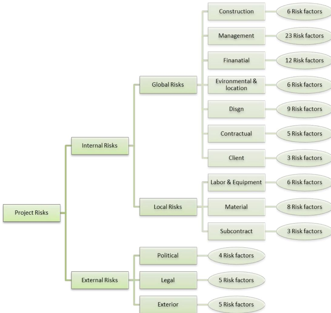
**Figure 02: Hierarchal Risk Breakdown Structure for the Project**
