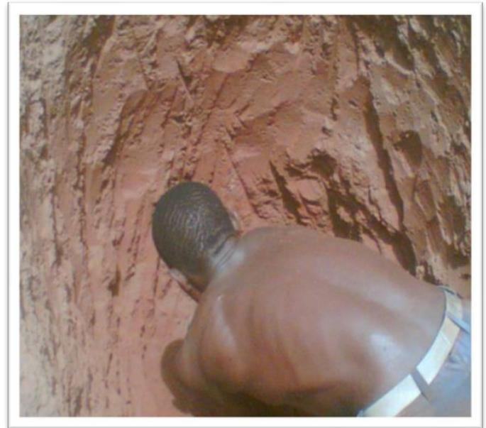
Figure 2: Sample Trial Pit dugged during Sampling Operations
