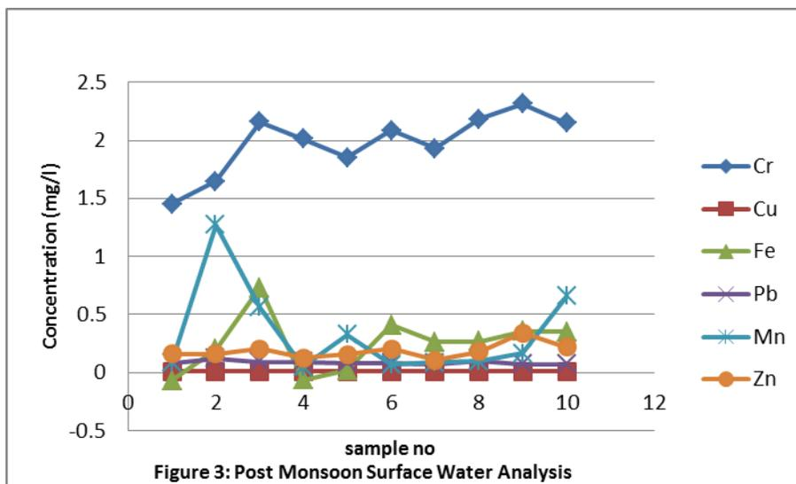
The flame type Atomic Absorption Spectrophotometer (AAS) analysis was done for heavy metals concentration of soil samples which was collected for different distances and depths of ground from the surrounding of disposal/dumping sites of study area is presented in fig. 3. The concentration obtained ( $Zn > Pb > Fe > Cr > Mn$ ) shows that heavy metals in the soil near the disposal/dumping sites is more and it is decreasing with respect to horizontal direction as well as with respect to depth also.
