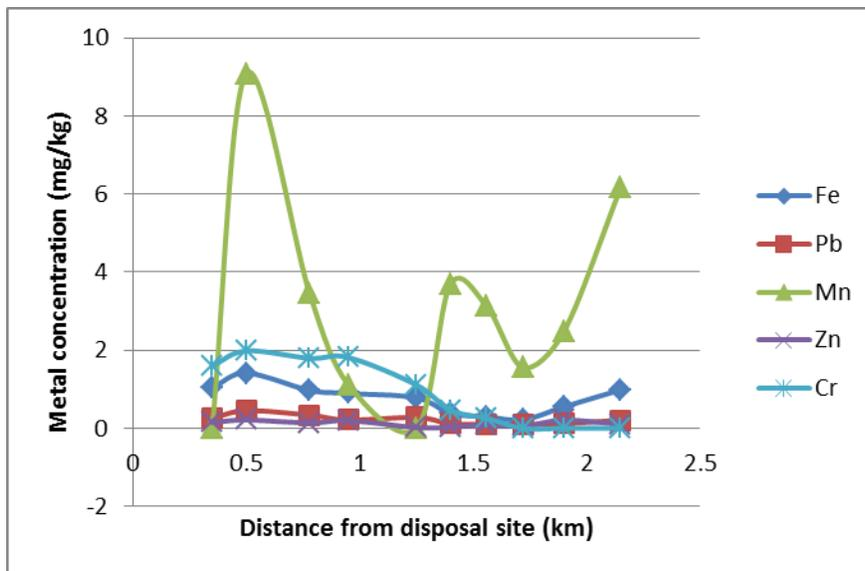
**Figure 4: Heavy metal concentration in soil (Distance wise sampling)**
