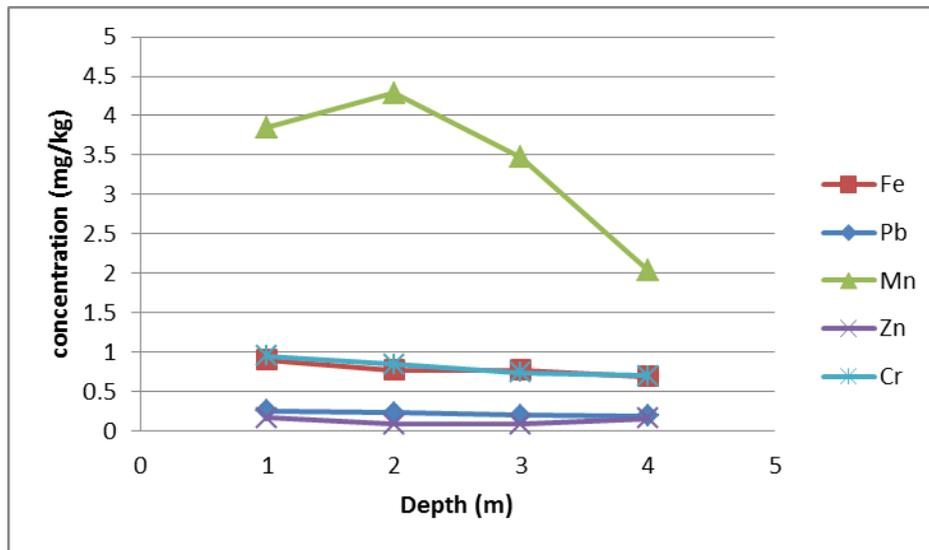
Figure 5: Heavy metal concentration in soil (Depth wise sampling)
