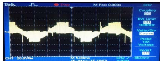
Fig 8(b) Waveform of phase to phase voltage (red-black) at speed 600 rpm.
