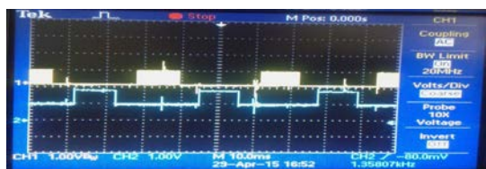
Fig 7(a) Waveform of PWM at speed 400 rpm.
