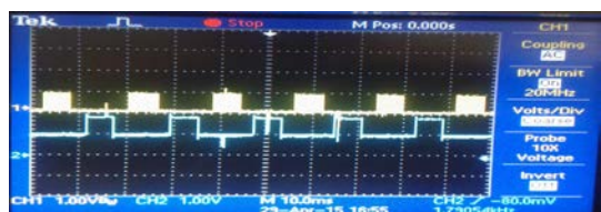
Fig 7(b) Waveform of PWM at speed 600 rpm.
