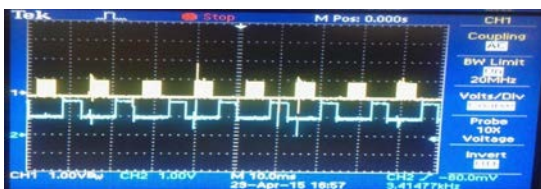
Fig 7(c) Waveform of PWM at speed 1000 rpm.
