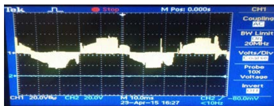
Fig 8(a) Waveform of phase to phase voltage (red-black) at speed 400 rpm.
