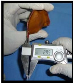
Fig 6 Thickness is measured with caliper
