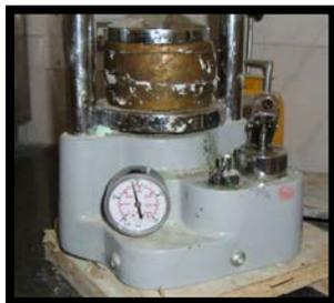
Fig 7 Bench curing at 3000 psi in Bench press
