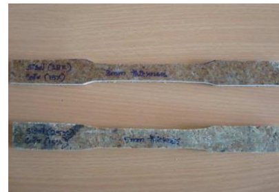
Figure 4.1.1 Specimen plate with 25% of sisal and 15% of coir
