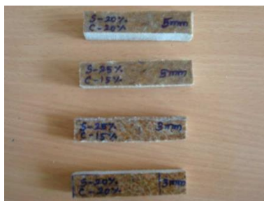
Figure 4.3.1 Specimen for impact test
