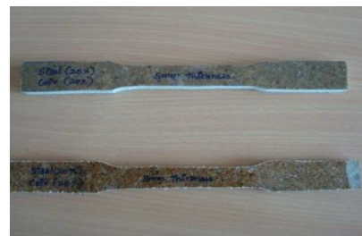
Figure 4.1.2 Specimen plate with 20% of sisal and 20% of coir
