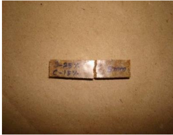
Figure 5.3(a) Specimen after Impact Test
