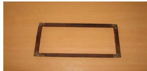
Figure 3.1 Moulds for Making Composite Plates
