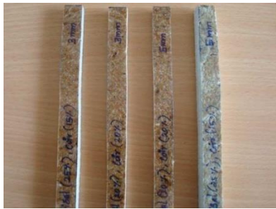
Figure 4.2.1 Specimen for flexural test
