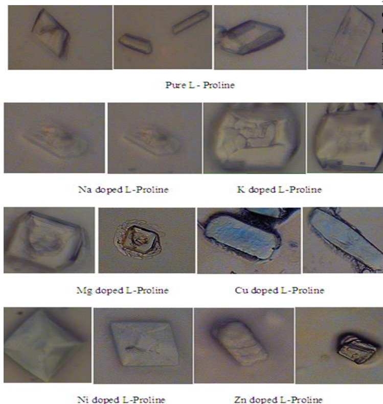
Fig.6 Surface revealing of etched pure and metal ions doped L-proline single crystals
