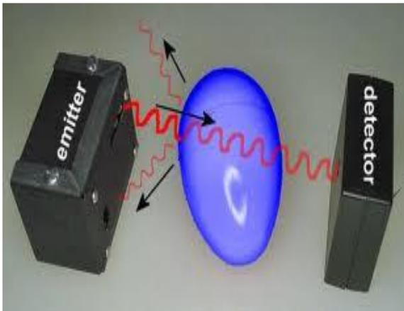
The seat belt is placed between the IR emitter and detector . The seat belt is teared horizontally at the center after leaving some length this helps to receive IR rays from the emitter by the detector to complete the circuit and it is encoded to RF circuit it converts it into radio frequencies . the radio frequencies are transmitted through antenna.
