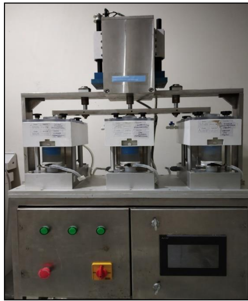
Fig.01 Accelerated pulsative valve tester
