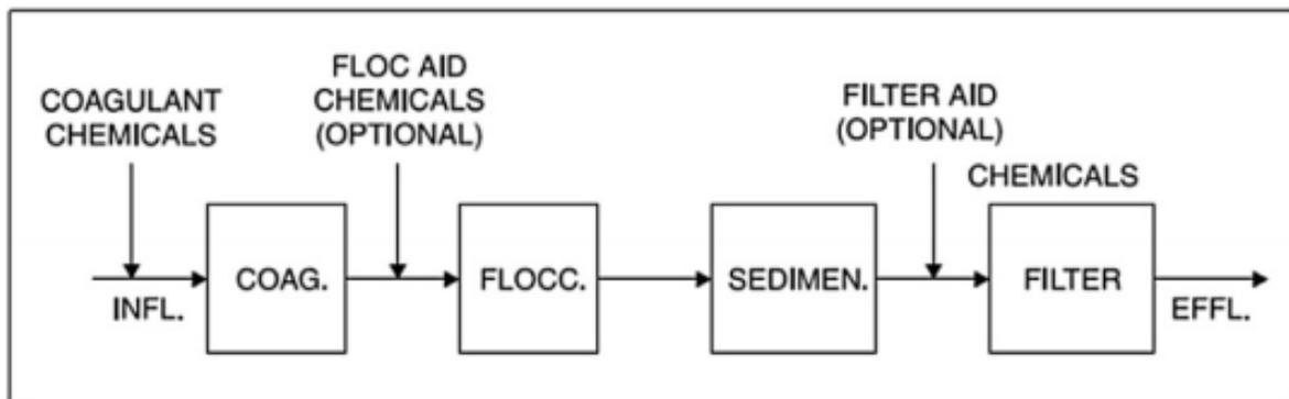
**Figure 6** Schematic diagram of conventional filtration processes at Zomba and Liwonde water treatment plant. INFL-Influent, EFFL- Effluent, COAG- Coagulation, SEDIMEN- Sedimentation, FLOCC- Flocculation. Source (Manda, Chidya et al. 2016)
