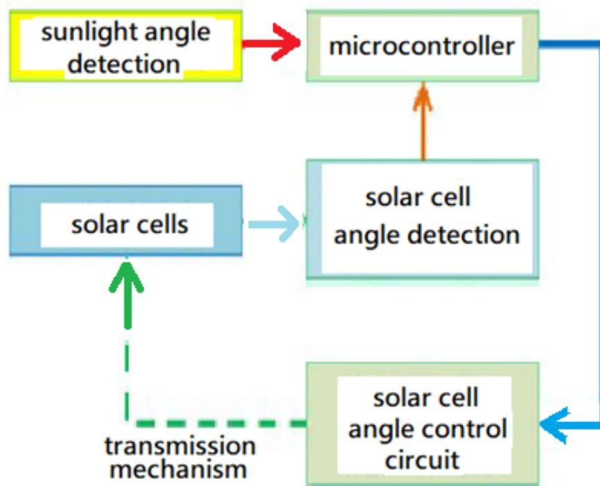
Figure 3: Vertical wall type solar photovoltaic system hardware structure diagram
