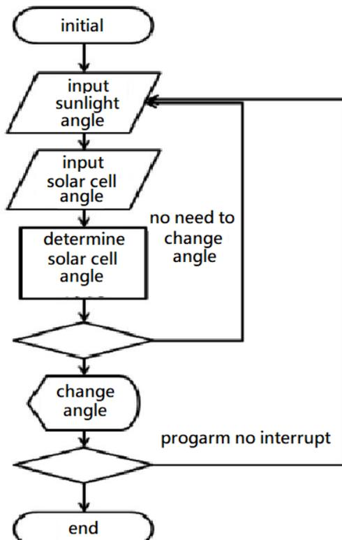
Figure 4: Vertical wall-to-light solar photovoltaic system control program flow chart
