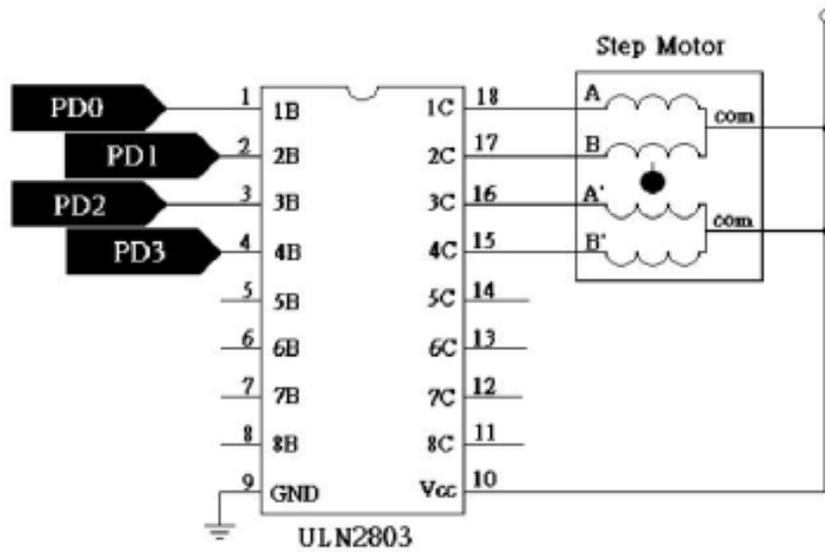
Figure 7: PD0 to PD4 pin connection of HT66F50 ULN2803 and stepper motor
