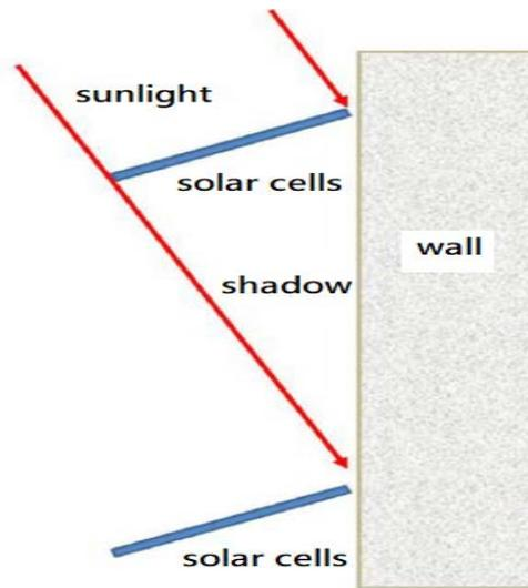
Figure 1: Solar panels on the wall to consider the effect of shadow
