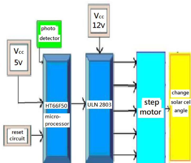
Figure 5: Overall composition block diagram
