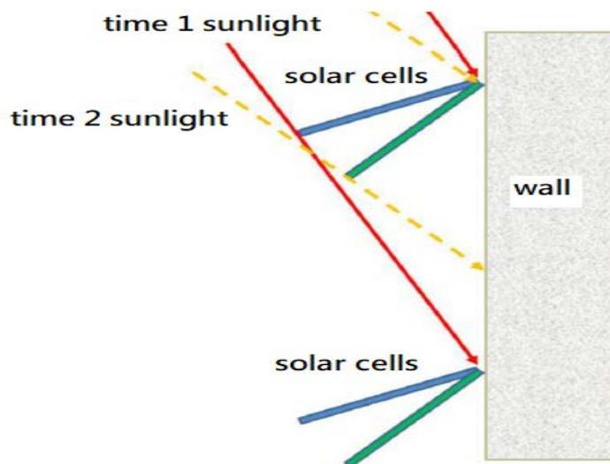
Figure 2: Solar panel tilt angle adjusted with sun angle
