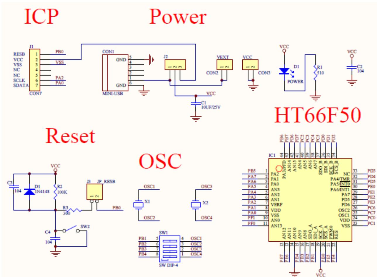
Figure 6: Reset circuit connection diagram of HT66F50
