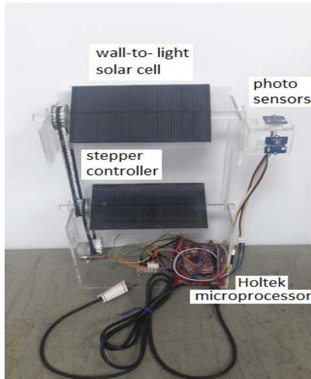
Figure 10: The finished wall-to-light circuit
