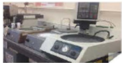
Figure 8: Motopol 2000 Struer auto polishing machine for metallographic preparation.
