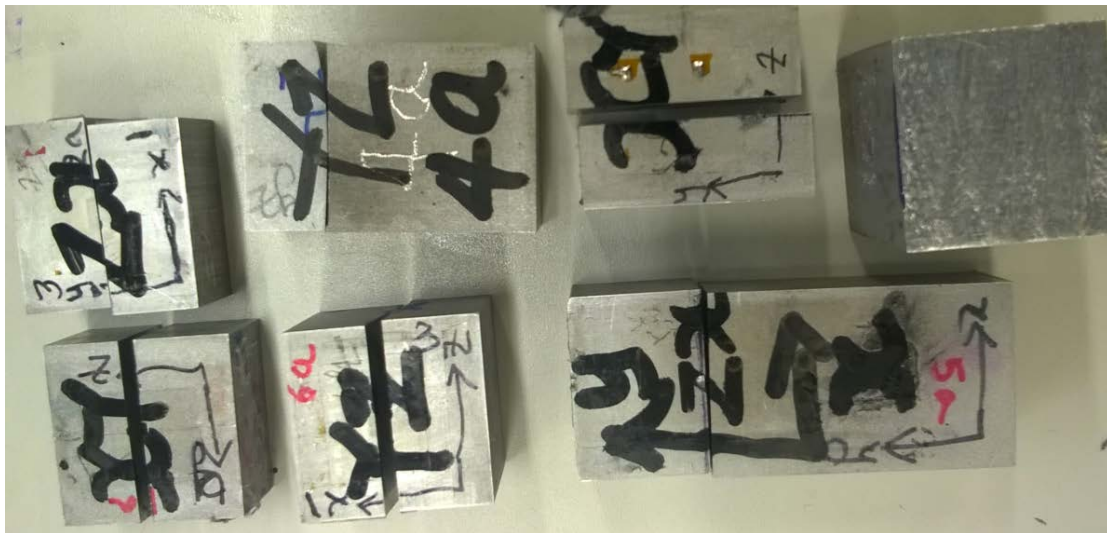
Figure 7: Al 2099 specimens for hardness test marked and sectioned along the drilled hole.
