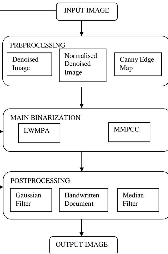
Fig.2. Flowchart of the proposed binarization method.
