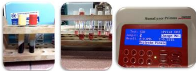
Figure 1. Separated Serum After Centrifugation (left), and Glucose Determination using Glucose Oxidase Method (middle and right)
