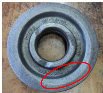
Photograph 1: Unfilling defect at front side of job
