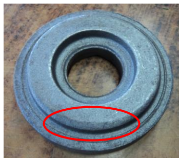
Photograph 2: Unfilling defect at back side of job
