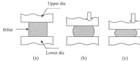
Figure 1: Open-die forging
