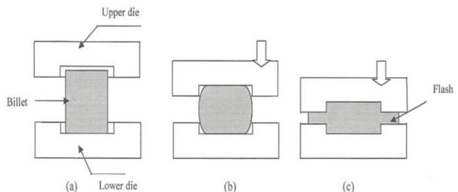
Figure 2: Impression-die forging
