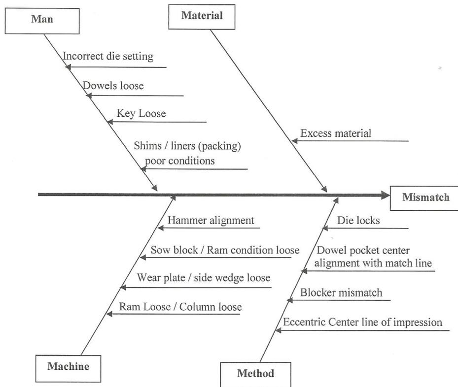
Figure 7: Fish-bone diagram for root-cause analysis of mismatch defect.
