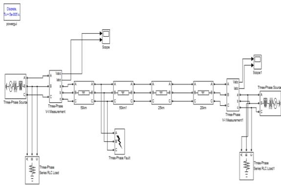
**Fig 3. Simulation model of single line diagram**
