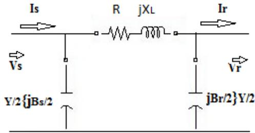
**Fig. 1 Pi-Network for a Transmission Line Model**
