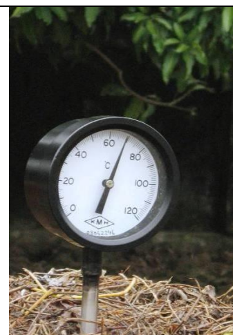
Pic. 3: Regular monitoring of temperature of Novcom compost heap ensures compost quality.
