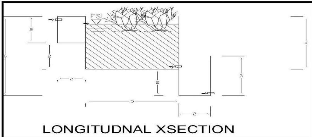
Fig-3: Macrophytes Stabilization Pond (Section)
