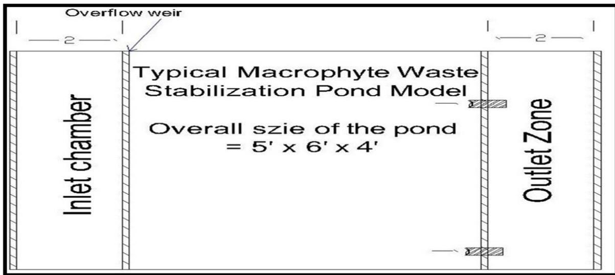
Fig-2: Macrophytes Stabilization Pond (Plan)
