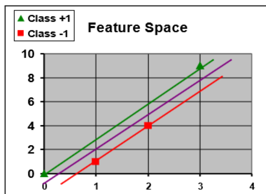
Figure 5: Simple Data in a Feature Space Separated by a Hyperplane
